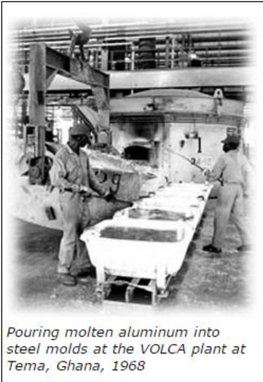
*Pouring molten aluminum into steel molds at the VOLCA plant at Tema, Ghana, 1968*
